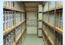
The MERLIN cluster 180 Dual AMD MP2200 1 GB RAM per node Albert Einstein Institute Golm, Germany
