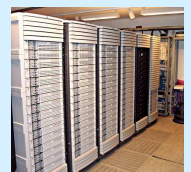
Lucidor cluster 90 Dual Itanium2 900 MHz 6 GB RAM per node Center for Parallel Computers, Sweden
