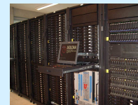
IITAC cluster , top500.org 356 opterons, 80 zeons Trinity Centre for High Performance Computing, University of Dublin, Ireland
