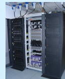
Genome research cluster 168 IBM HS20 Blades 2x2.8 GHz P4 The Sanger Institute Cambridge, UK
